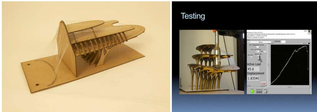
Figure 7: Boat concept applied to building form and model test with corresponding load-deformation curve
