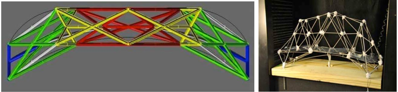
Figure 2: Computer simulation of distribution of internal forces and the actual load-test of the model
