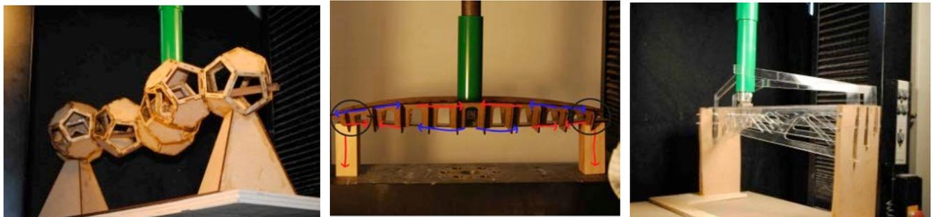
Figure 3: (a) Poluhedral modules, (b) Bowed vierendeel and (c) Doble cantilevererd system
