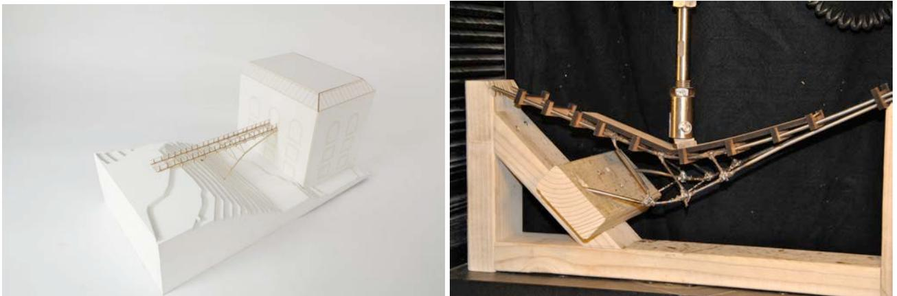
Figure 5: Site model and load-test of the pedestrian bridge
