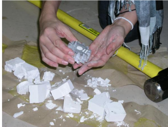
Figure 7. Breaking the mold to obtain the casting
