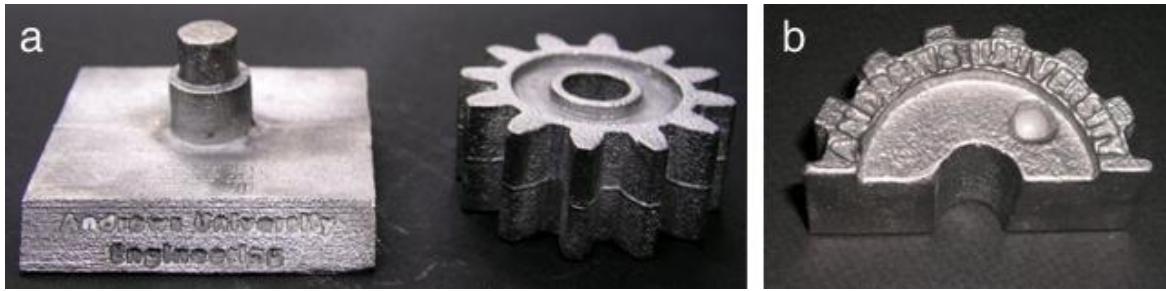
Figure 9. The casted products, a) gear and mounting for the gear stand combination set and b) the half gear.
